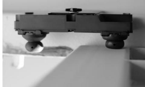
Close the left door. Make sure that the left "rubber boot" on the unit is compressed with the left door as shown. The unit is now correctly installed\* and the container doors can be sealed for transport.
